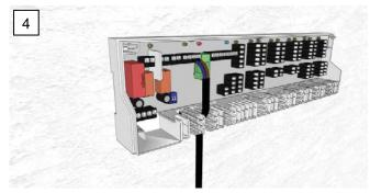
Lay the cables into the casing through the strain relief and install all cables to the basis using the clamping/plug-in technology; this is possible in a very short time.
