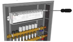
Loosen the casing cover at both latching points with a screwdriver and remove it.
